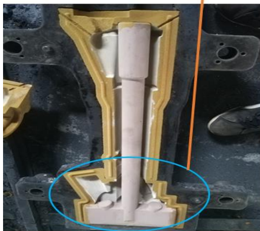
Fig 3: -Chills provided in sand mould of cylinder before molten metal pouring.
