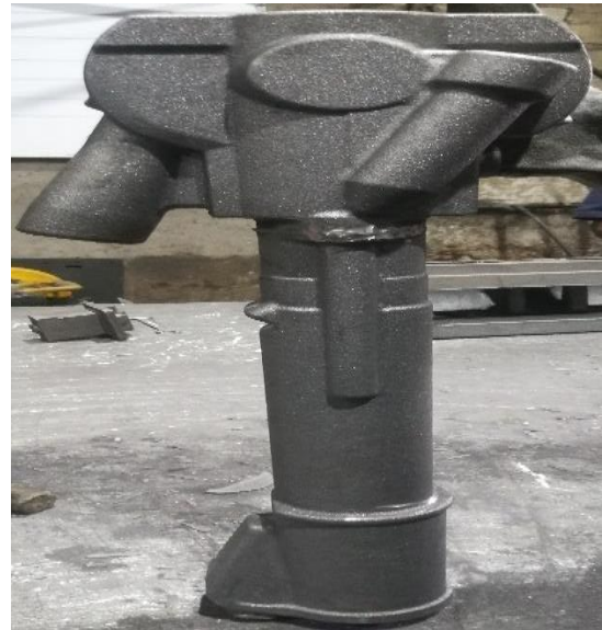
Fig 9: View of Finished Cylinder with Negligible Defect
