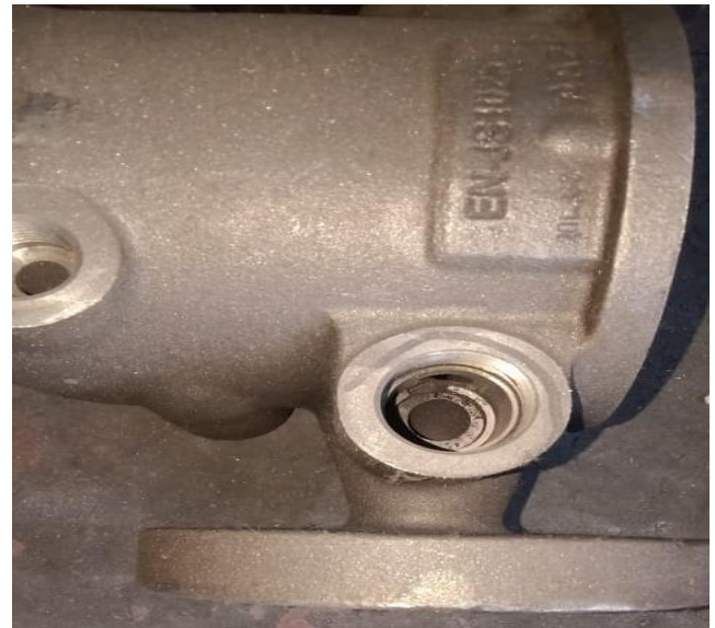
Fig 4: - Shows shrinkage defect in CMTOFT over
