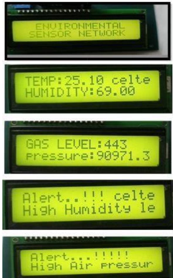
Figure 4: LCD Display for monitored results
