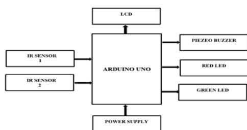
Fig 4: Passenger Counter block diagram
