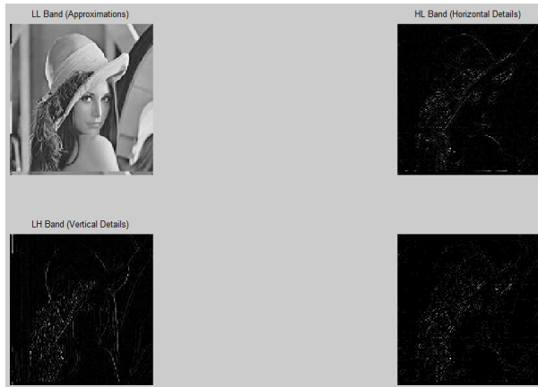
Fig. 10: Output of 2D-DWT Block
