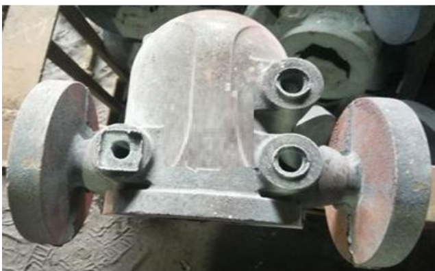
Fig 8: -CMTOFT cover after solidification
